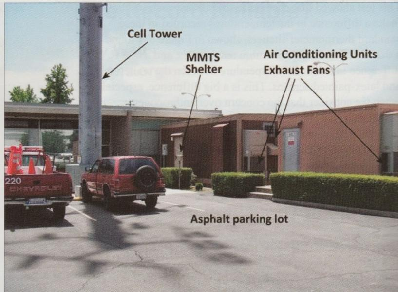
Figure 5. Temperature station at the Marysville, California fire department surrounded by heat sources.
